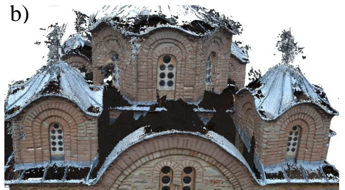
figure 7 - Textured point cloud from Close-range photogrammetry - details
