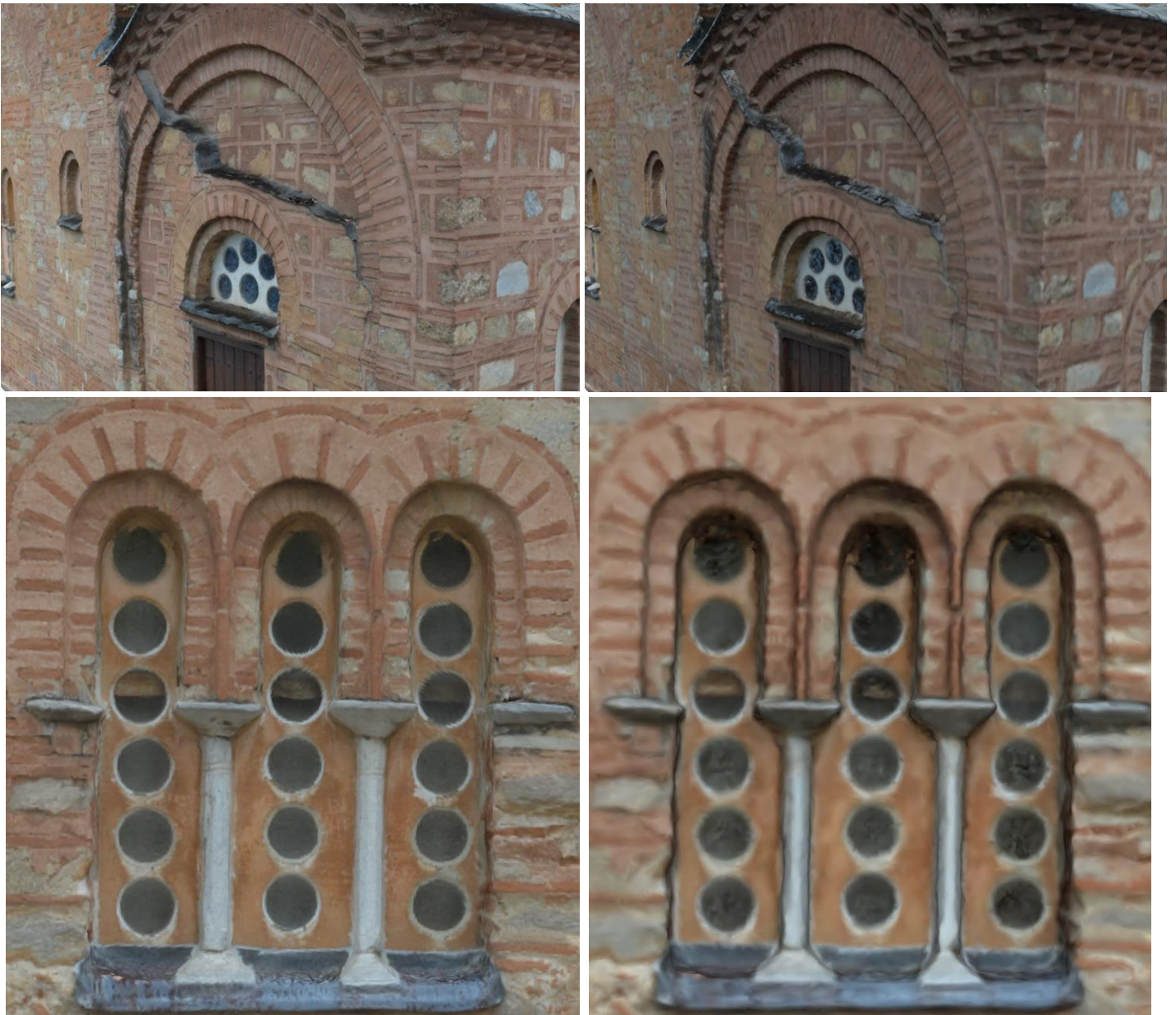
figure 22 - 3D model in detail - textured (left), mesh (right)
