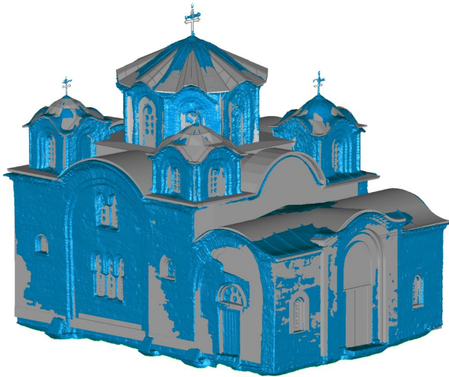
figure 35 - Comparison of the 3D models - BIM model (grey), reference photogrammetry model (blue)
