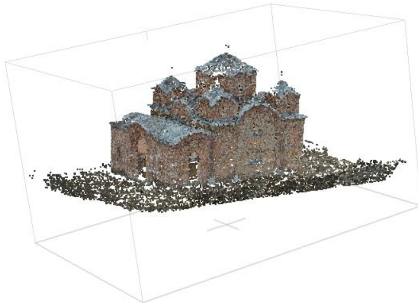
figure 18 - Cleaned' sparse point cloud
