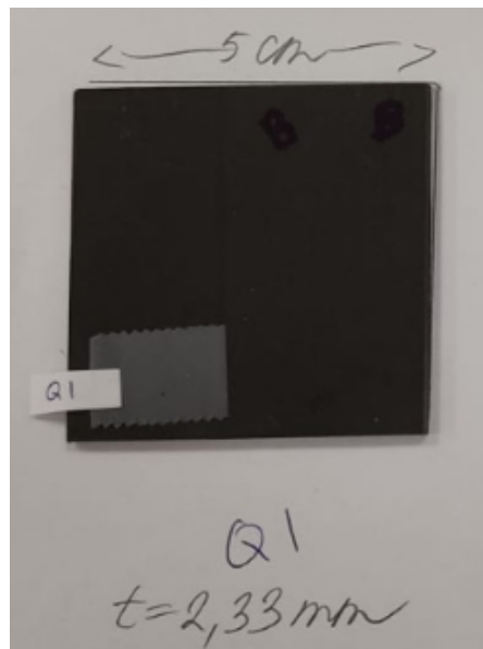
Figure 6.28: Sample Q1 used for measurements - Carbon Composite. Thickness of the sample is 2.33 mm and density is 1.54 \text{ g}\cdot\text{cm}^{-3} .
