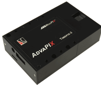
Figure 6.12: The TPX3 AdvaPIX radiation camera. Operation, control and readout require a single USB 3.0 connector/cable. Power is supplied by additional/separate DC +5 V connector/cable.
