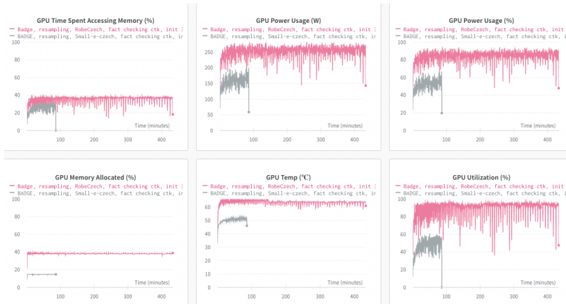
Figure C.3: Illustration of several system parameters (GPU state) that are natively supported by Weights & Biases and that are automatically monitored during each experiment. GPU utilisation charts help to figure out how the hardware is capable of processing large batches and store large models in GPU RAM.
