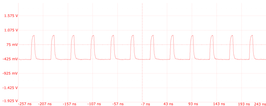
Figure 7.2: Fits LVDS channel voltage at FPGA termination.
