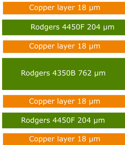
Figure 4.14: Used Rogers material board stackup.
