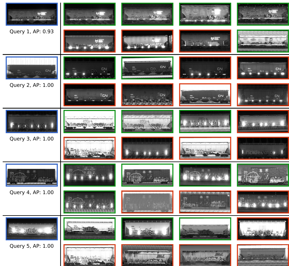
Figure 4.5: Example of top-8 retrieval results for query car images with unique drawings and graffiti. The retrieved samples are sorted by the euclidian distance from the query descriptor from top to bottom and left to right.
