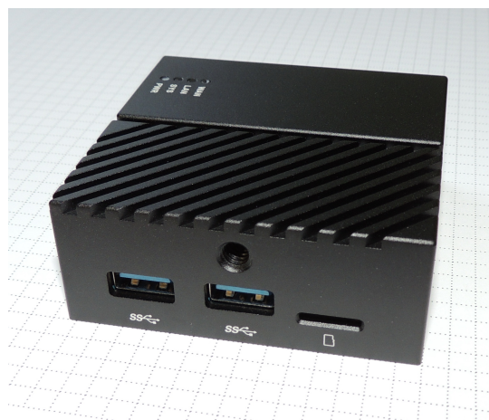
(b) USB 3.0 ports, MMC slot and 1/4" camera screw thread
