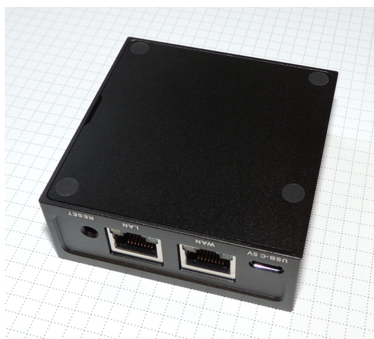
(c) Ethernet ports, USB-C and Reset button
