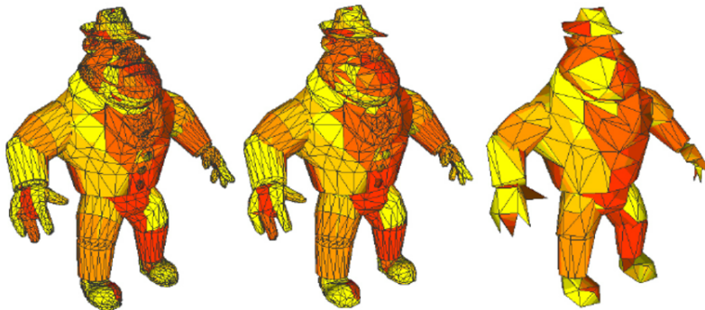
Figure 2.3: A model captured with 3 different LODs. (Source: [26]).
