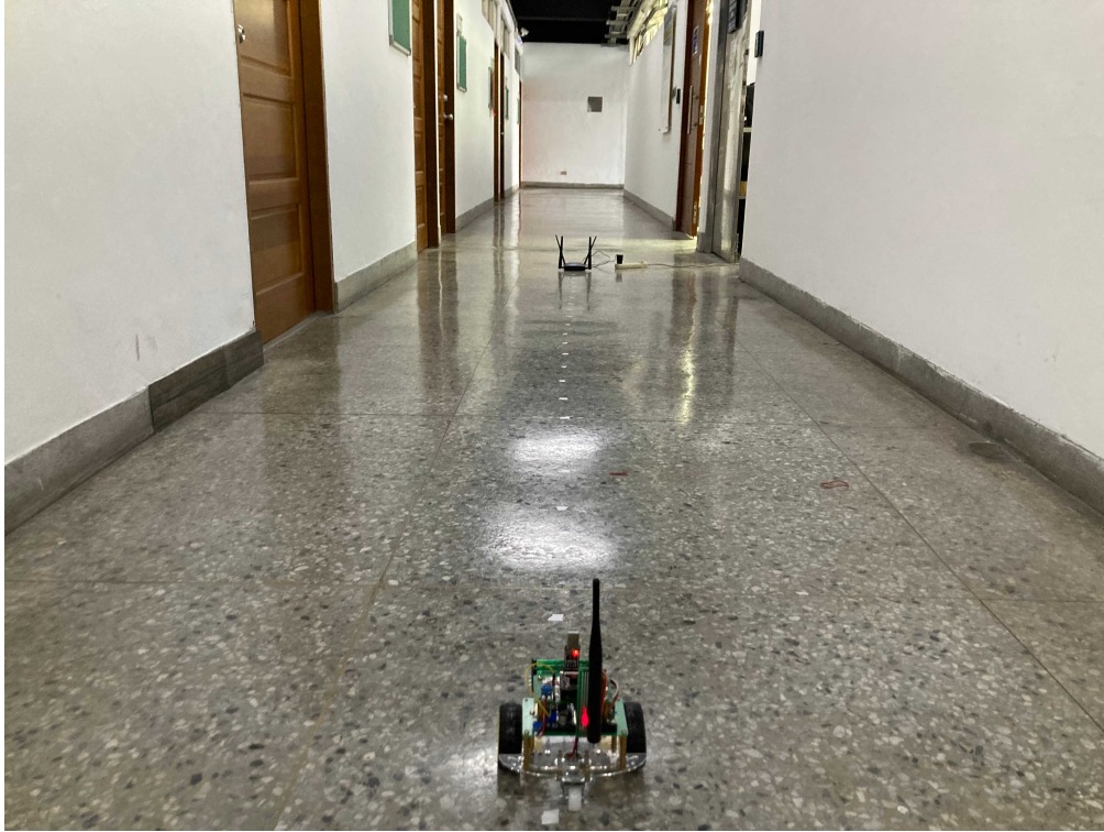
Figure 4.2: Experimental setup of the RSS measurement in a school hallway.
