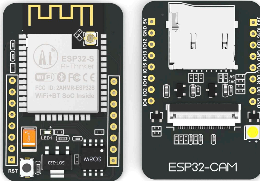
Figure 3.7: ESP32-CAM (AI-Thinker module). Image acquired from [11].
