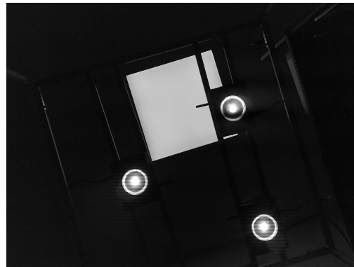
(b) Image with tuned camera parameters for showing LED's fingerprints on the image.
