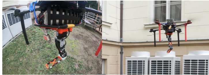
Figure 4.6: Flying UAV with the attached manipulator [left = camera mounted on UAV, right = view from ground]
