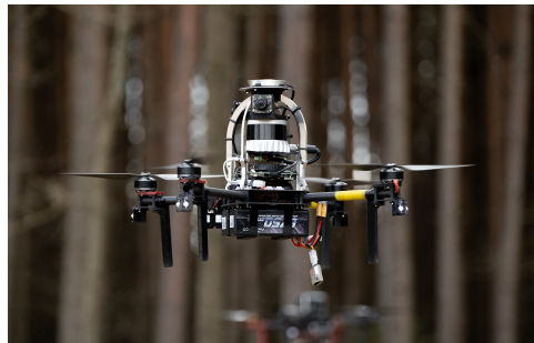
Figure 1.2: Example of an MAV quadcopter equipped for science purposes - Holybro X500 used by MRS group at CTU.
