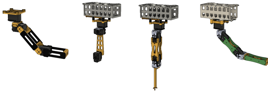
Figure 2.7: Manipulator design iterations. Oldest (left) to current (right).
