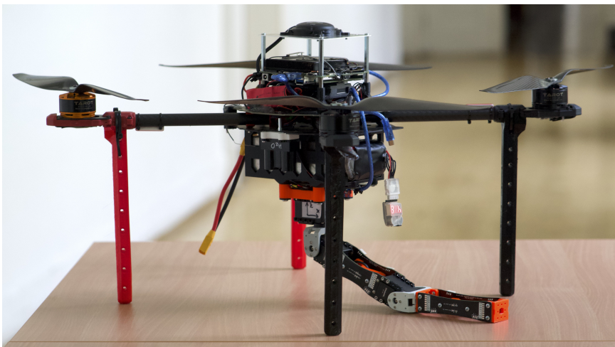
Figure 4.4: Side view of the manipulator attached to Tarot T650 Sport UAV
