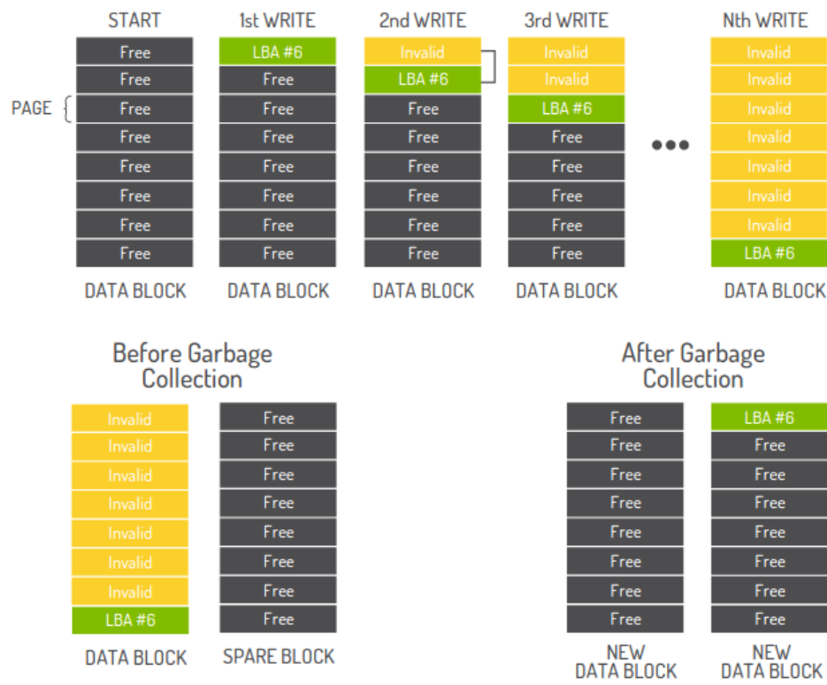
Figure 3.1: Dynamic wear levelling[42]
