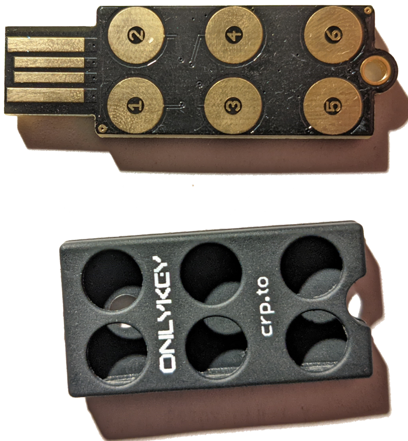
Figure 1.6: The OnlyKey Color with the supplied cover removed from the front
