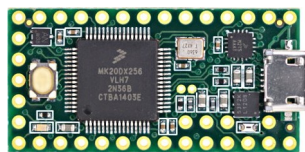
Figure 1.1: The Teensy 3.2 device front (downloaded from the PJRC website[6])
