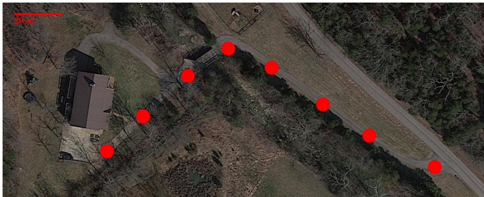
Figure 4: Demonstrator communication infrastructure building mission result based on reactive 1 Hz RSSI measurements. The background image source: Maps Data: Google ©2023 Landsat/Copernicus.
