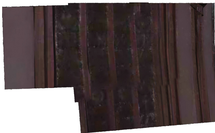
Figure 6.3: Image mosaics from captured images of simulation 1. There are not present all images captured. It is probably due to one row of images not being able to stitch to the others and thus disconnecting the rest.
