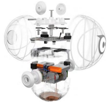
Figure 13 Inside the Sphero SPRK edition [11]
