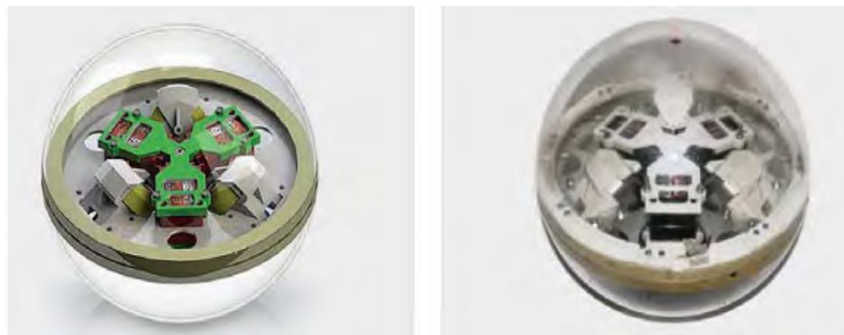
Figure 3 A 3D design (left) and a full-scale photograph (right) of the design of the robot with 3 rotors [1]
