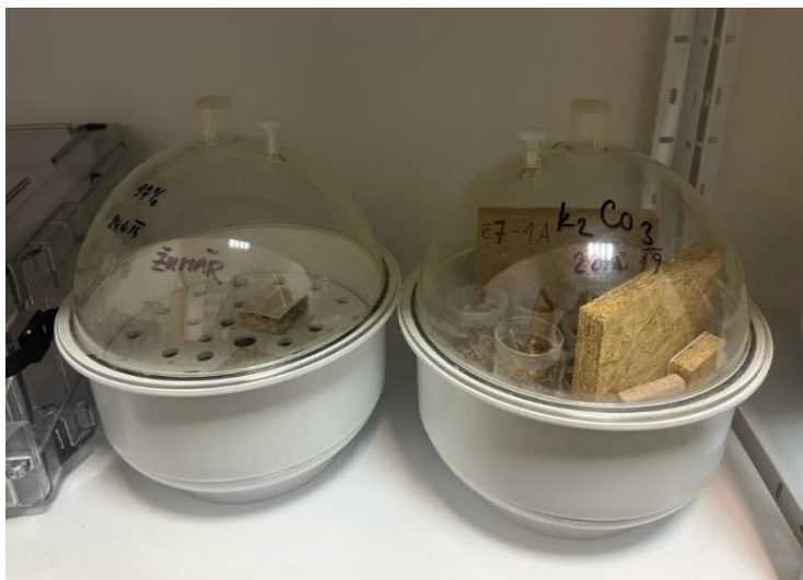
Figure 10: Samples were conditioned inside 97% of salts and Potassium Carbonate.
