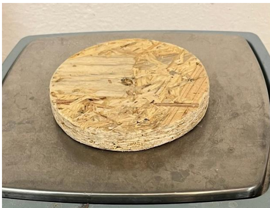
Figure 19: OSB board without coating before abrasion test.
