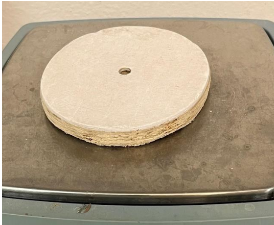
Figure 18: OSB board with coating before abrasion test.
