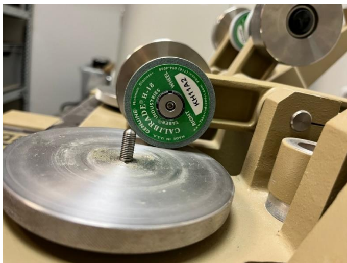
Figure 20: Picture shows calibrating wheels. Test was done by calibration method. Medium grain, medium abrasion, grey, vitrified, sintered serves as a medium-coarse abrasive. It is most frequently used to assess durable materials like flexible plastic sheets, woven textile fabrics, coated fabrics, and rubber that isn't sticky.
