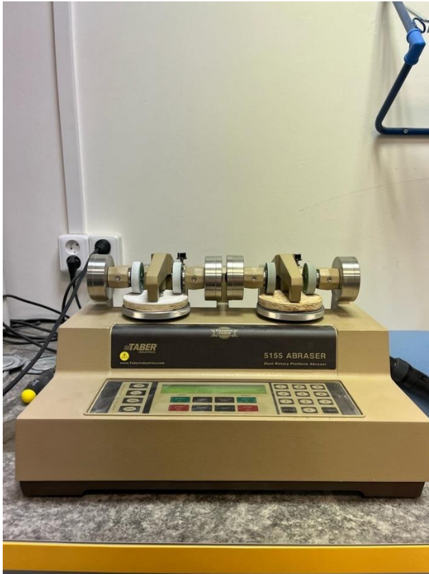
Figure 21: Two samples are being abraded in the machine.
