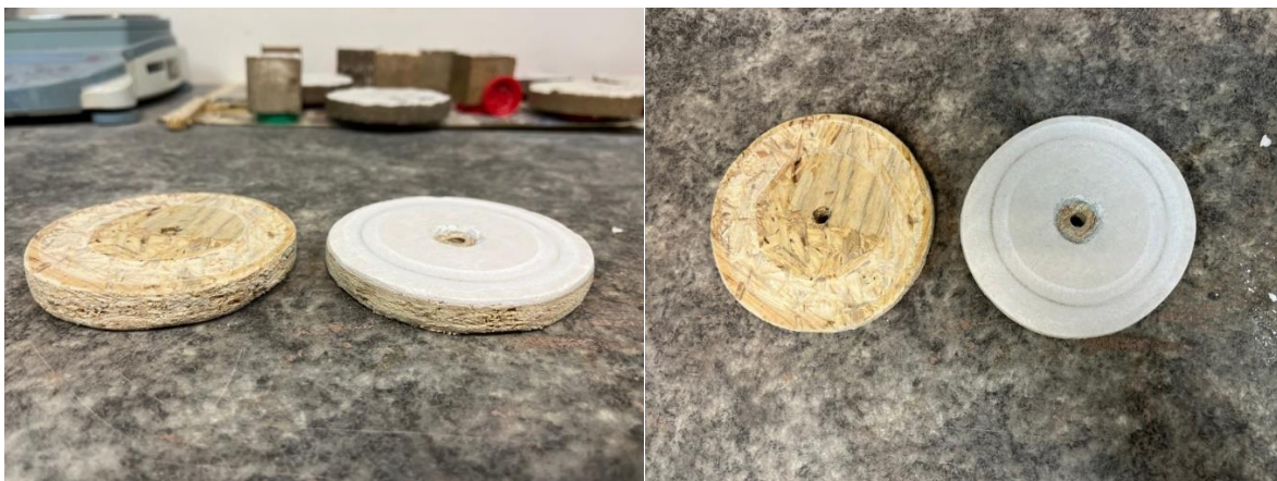
Figure 22: Samples after the abrasion with 3000 rotations.
