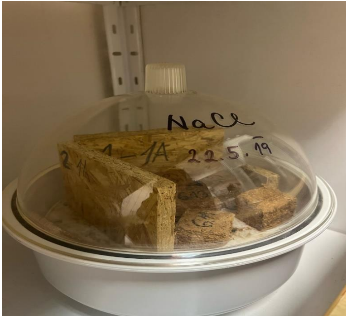
Figure 12: Samples are inside of the box of Sodium Chloride
