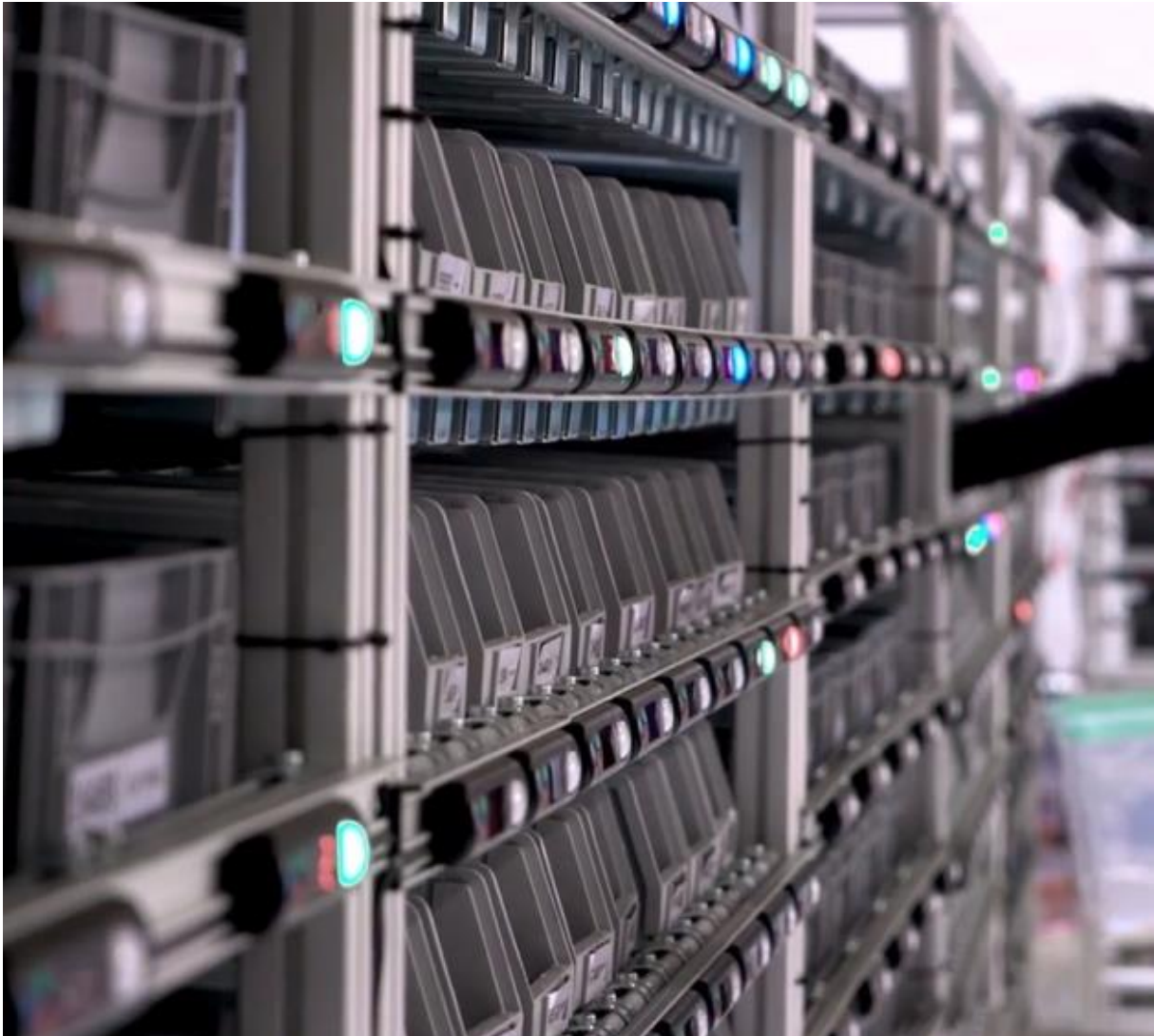
Figure 1: Pick-to light systems. [2]
