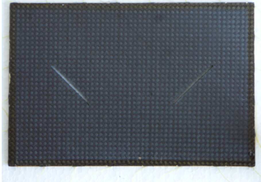
Figure 6.2: Set of CFRP specimens (A). One specific specimen of dimensions 150 \times 100 mm with defects (B) of the length of 35 mm positioned at coordinates X: \pm 37.5 mm; Y: 0 mm at an angle \pm 45^\circ with a width of 1 mm.
