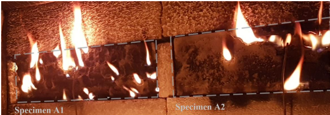
Figure 12: Plate specimens without polypropylene fibres after the fire test
