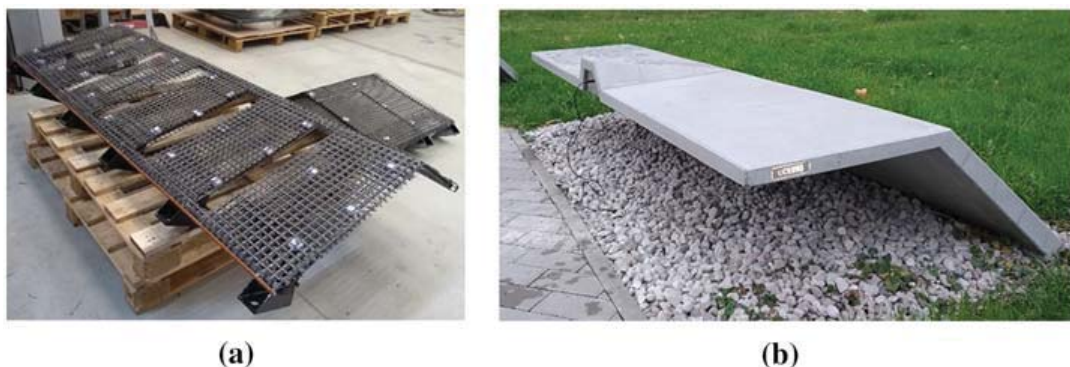
Figure 1. Example of the reinforcement mesh and structures made out of TRC: (a) carbon fiber reinforcement in the form of an L-angle with impregnation from the epoxy resin; (b) example of non-load-bearing structures made out of textile-reinforced concrete.
