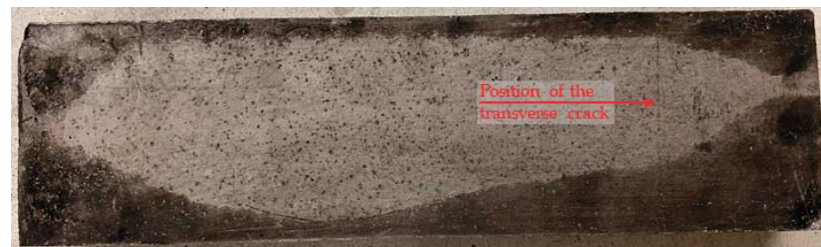
Figure 8. Test specimen with 10 mm covering layer and an addition of PP fibers in concrete mixture (HPC mixture No. 1)—the development of a transverse crack during a fire test.
