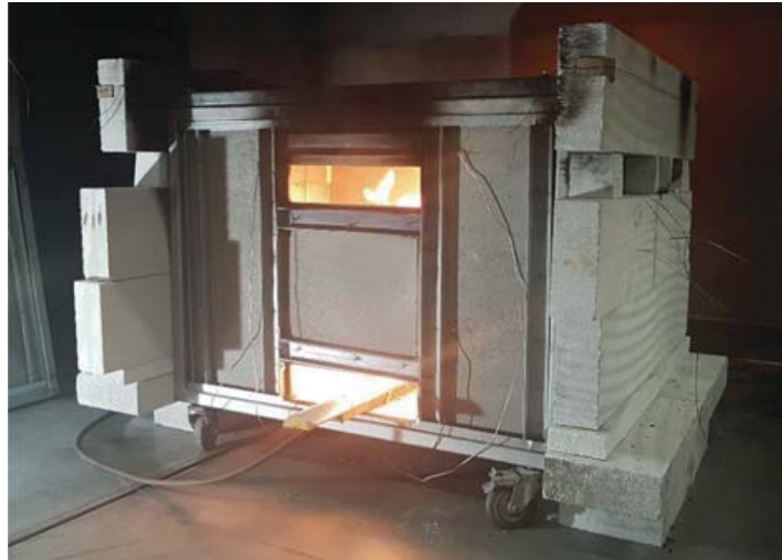
Figure 11. Medium-scale fire furnace (miniFUR) during the indicative fire experiment.
