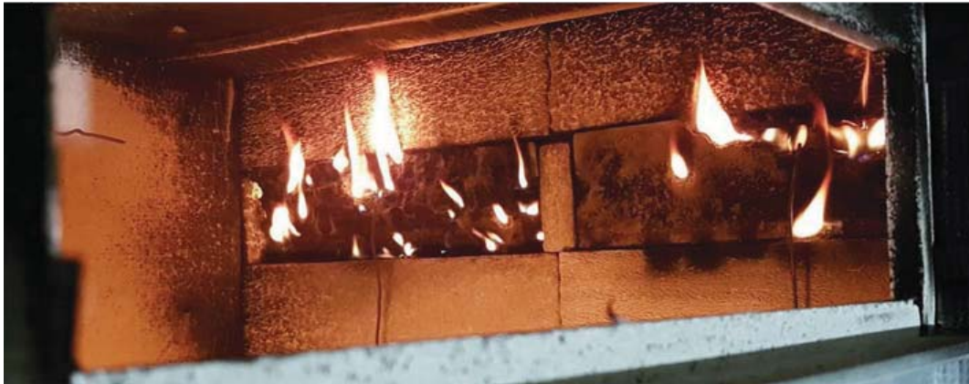
Figure 13. View through the ventilation opening of the experimental samples' burning surface in the furnace: ignition of C-sample, without PP fibers (left) and D-sample with PP fibers (right), after the end of the indicative experiment.
