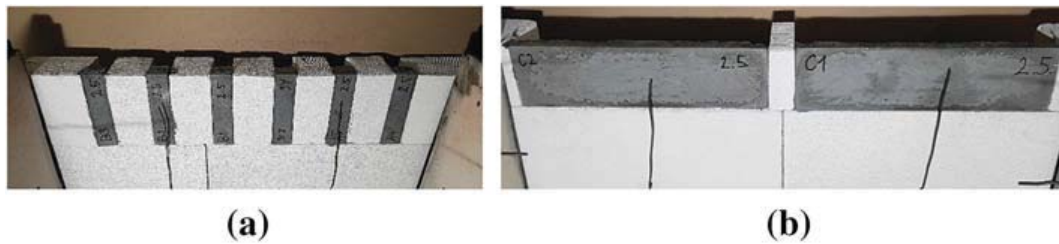
Figure 7. Attaching of experimental samples to the front wall of the concrete brick furnace: (a) beam samples; (b) plate samples.
