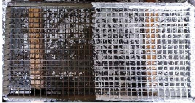
Figure 7. Preparation of reinforcement mesh: (a) Method of carbon mesh preparation (unit: mm); (b) Mesh from carbon roving saturated with cement suspension—surface application by roller (from left): CEM 42.5 R, CEM 52.5 R.
