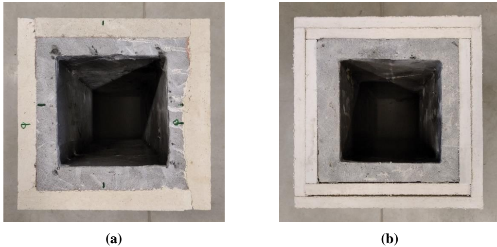
Figure 5: Variants of applied fire protection systems on a TRC hollow section column: (a) functional sample of a TRC column with gypsum plaster [36]; (b) functional sample of a TRC column with calcium-silicate boards [37]
