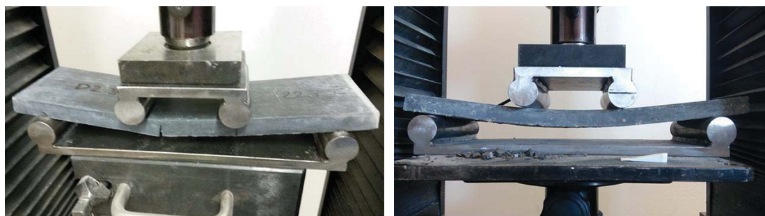
Fig. 7 – Typical crack development of 2x5 reinforcement with smooth surface on the left and 4x10 reinforcement treated with fine-grained silica sand on the right side.
