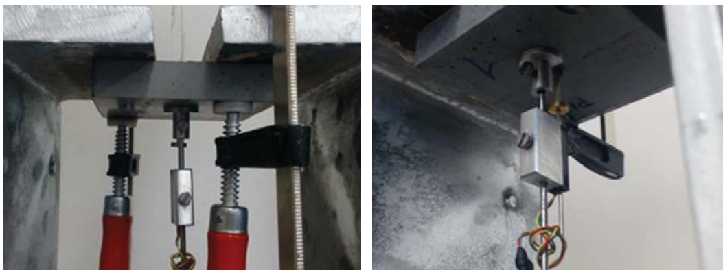
Fig. 4 – Detailed view of the bottom part of the concrete specimen with installed potentiometer and support constructions for the pull-out values measurement.
