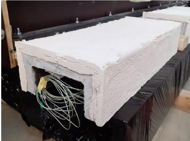
Figure 22: One of the specimens with gypsum plaster for the indicative fire test
