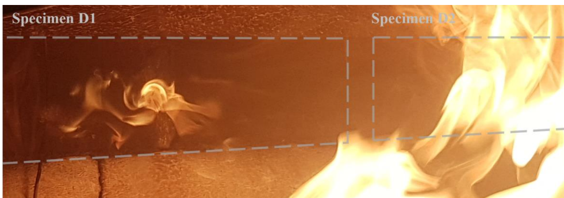
Figure 13: Plate specimens with polypropylene fibres during the fire test
