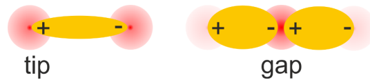
Figure 2: Illustration of electric field intensity in plasmonic hot spots: sharp tips and narrow gaps between the nanoparticles.
