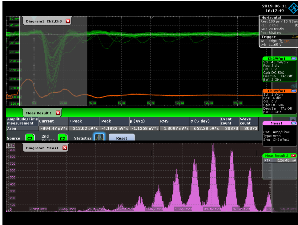
Figure 7.29: Waveform and collected spectrum of response to very low illumination by UV LED measured for Hamamatsu MPPC S12572-010P before irradiation. Signal from the SiPM is connected to Channel 2 (green) and trigger from the pulser is connected to Channel 3 (orange). Scale of horizontal axis is 20 ns/div, vertical is 40 mV/div for signal and 1 V/div for trigger. Measurement histogram on the bottom has horizontal axis with 0.47 nV-s/div, vertical axis shows arbitrary values due to oscilloscope software bug. Overvoltage is 3 V.
