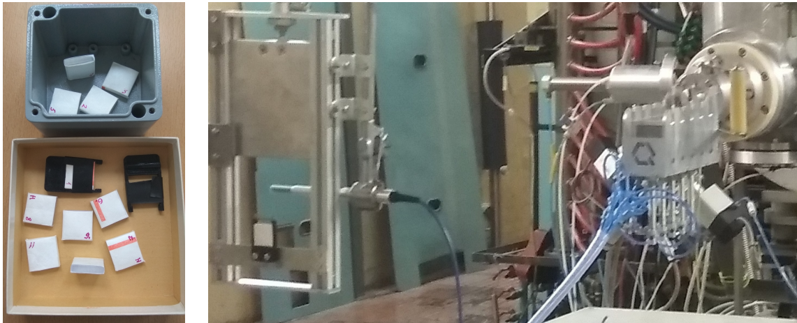
Figure 6.11: Scintillator samples prepared for measurements after the irradiation (left) and fixed at the cyclotron holder together with the ionization chamber (right).
