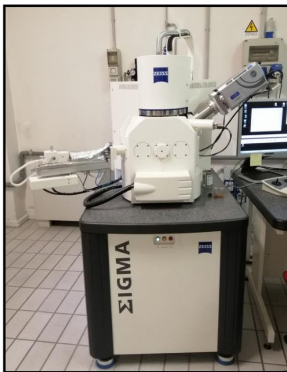
Figure 2-1 Zeiss Sigma FE-SEM 300 used in this work for the surface characterization of the Tm:Y 2 O 3 transparent ceramic samples.
