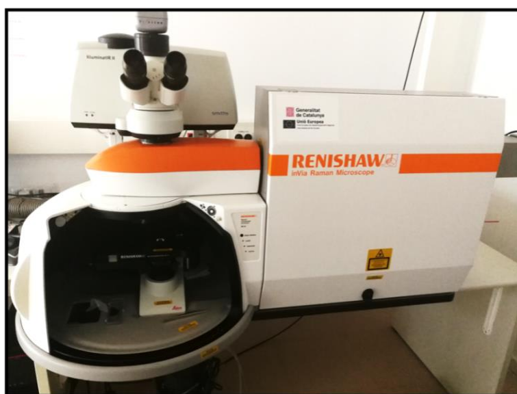
Figure 2-3 Renishaw in Via confocal Raman microscope used in this work for the vibrational characterization of the Tm:Y 2 O 3 transparent ceramic samples
