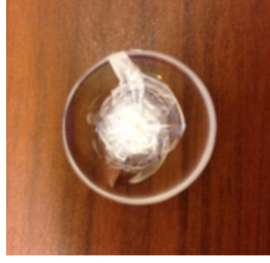
Figure 2.15: Laser induced optical damage in a laser window caused by high laser fluence.
