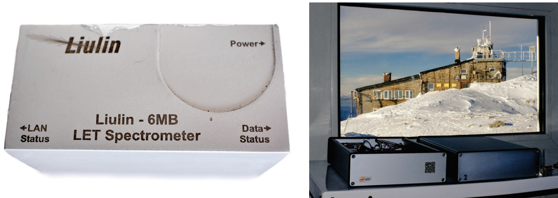
FIGURE 1. Liulin 6MB (left) and two AIRDOS units (right) installed at BEO Moussala
