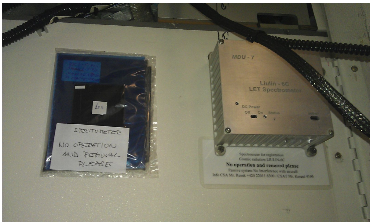
Figure 4: Liulin dosimeter (right side) deployed on board aircraft together with nuclear emulsions and TLDs (ThermoLuminescent Dosimeters) (left side). Courtesy of Czech Airlines.
