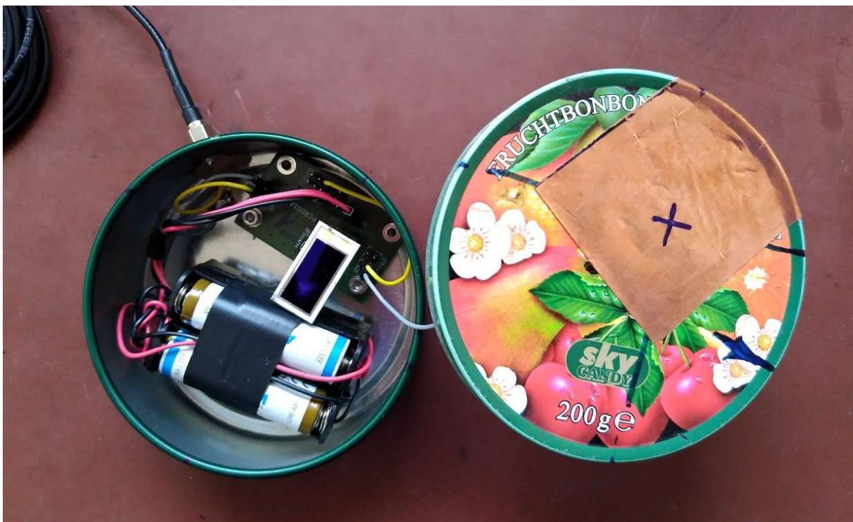
Figure 34: CANDY detector - mechanical setup. Please consider the size of AA batteries in order to imagine the dimensions.
