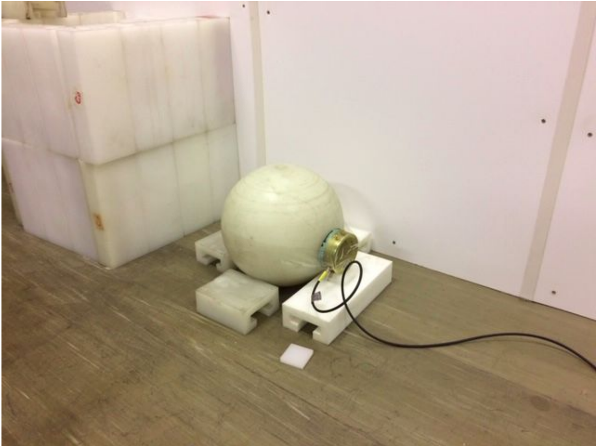
Figure 60: Irradiation of CANDY detector with an AmBe source placed inside HDPE sphere 300 mm in radius.
