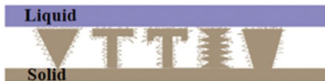
Figure 4: Illustration of overhang and re-entrant microstructures covered with nanoscale features [22].
