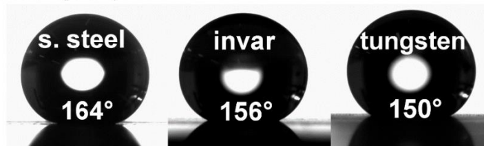
Figure 8. The wettability measurements of laser processed samples after vacuum treatment.
