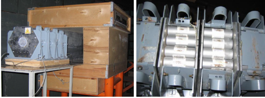
Figure 5: E+T setup with the biological shielding (left) and view of the uranium blanket (right) [47].
