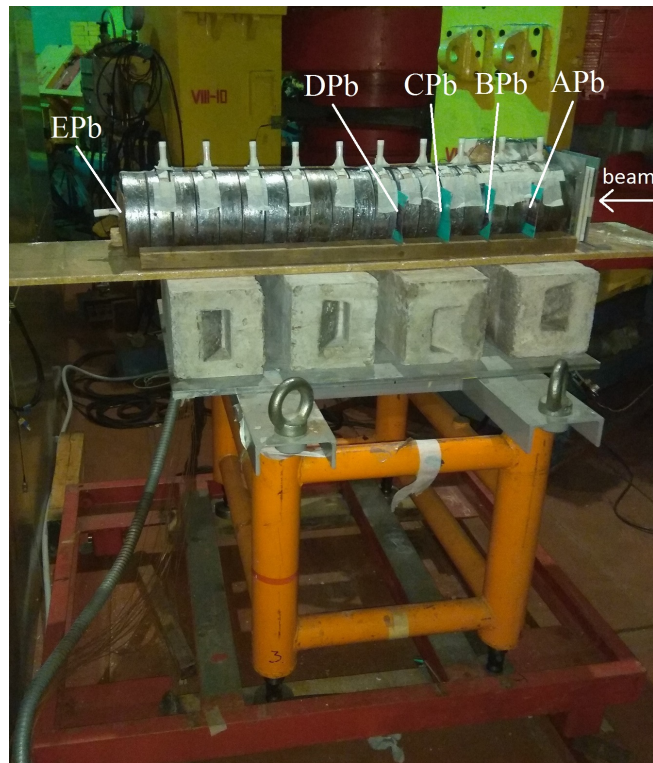
Figure 70: Lead target with its stand. The proton beam hits the target from the right side. The locations of the ^{nat}\text{Pb} activation samples are marked.
