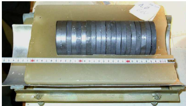
Figure 1: GAMMA-2 setup: lead target and part of its paraffin moderator [43].
