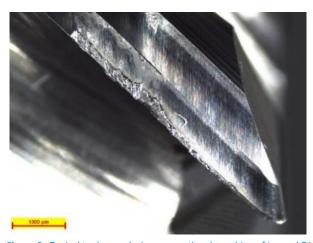
Figure 6. Typical tool wear during conventional roughing of Inconel 718
