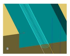
Figure 3. Proposed trochoidal toolpath for milling
