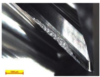
Figure 8. Typical tool wear during trochoidal milling of Inconel 718
