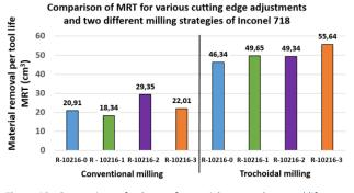
**Figure 10.** Comparison of volume of material removed per tool life (MRT) for various cutting edge adjustments and two different milling strategies
