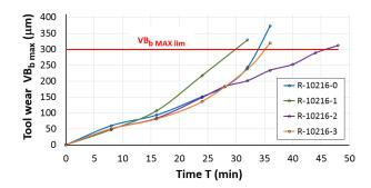
**Figure 7.** Graphical comparison of average VB<sub>b max</sub> wear characteristics for all tested tools when Inconel 718 conventional milling with cutting conditions:  $v_c = 40$  m.min<sup>-1</sup>,  $f_z = 0.06$  mm,  $a_e = 0.5$  mm,  $a_p = 4$ mm
