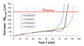
**Figure 9.** Graphical comparison of average VB<sub>b max</sub> wear characteristics for all tested tools when Inconel 718 trochoidal milling with cutting conditions:  $v_c = 40 \text{ m.min}^{-1}$ ,  $f_z = 0.06 \text{ mm}$ ,  $a_e = 0.5 \text{ mm}$ ,  $a_p = 4 \text{mm}$
