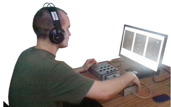
Figure 2. Measuring device used for collection of reaction times of tested subjects.
