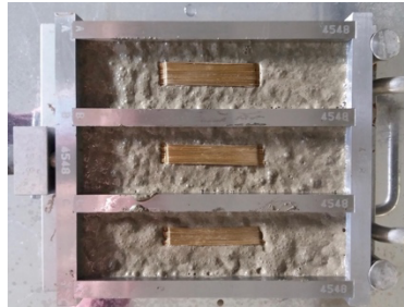
Figure 38. A mould for three 40x40x160 mm 3 specimens – a demonstration of the steel fibres placement.
