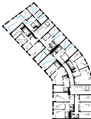
Figure 7 Apartment House Ostravská Brána natural ventilation schema on typical floor (1:1000) (source: author)
