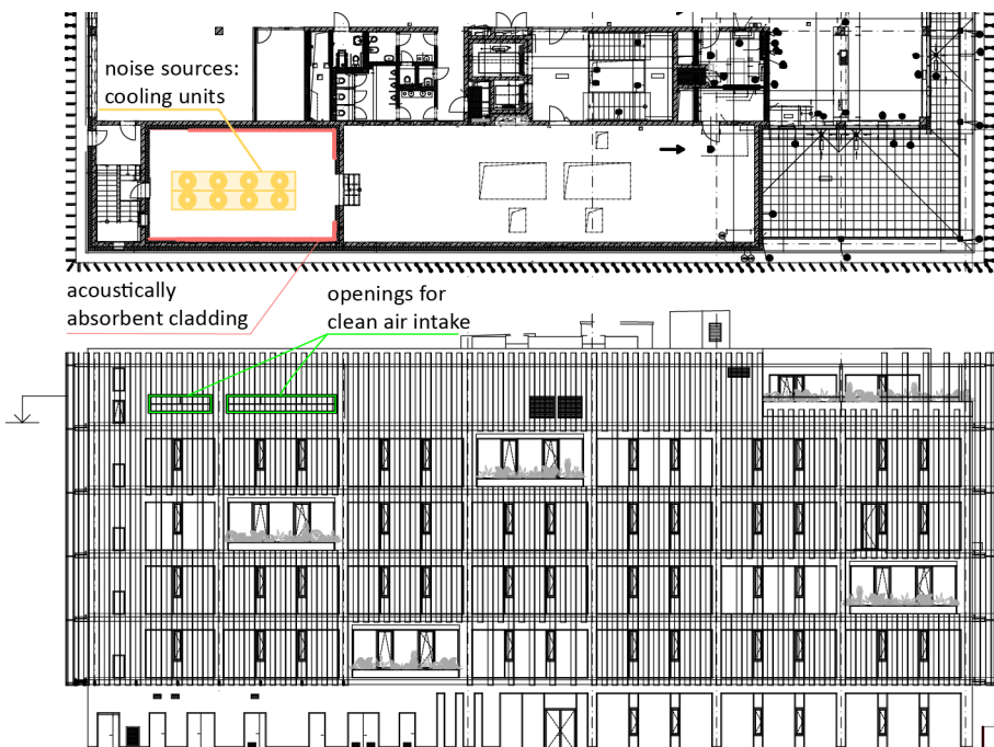
Figure 4.83 Office Building Konplan - acoustic treatment of noise sources on roof (1:500) (source: adapted from project documentation)
