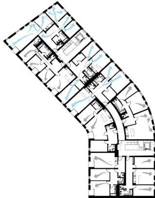
Figure 4.5 Apartment House Ostravská Brána natural ventilation schema on typical floor (1:1000) (source: author)
