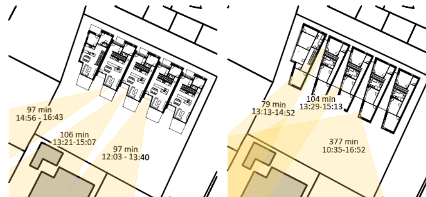
Figure 4.23 Terraced Houses Zruč sunlight provision on 1.3. on 1 st (left) and 2 nd (right) floor (1:1000) (source: author)
