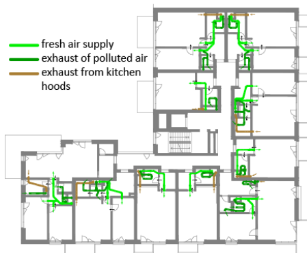
Figure 4.14 Residential Block 4BLOK mechanical ventilation on 2 nd floor, Block II (source: adapted from documentation)
