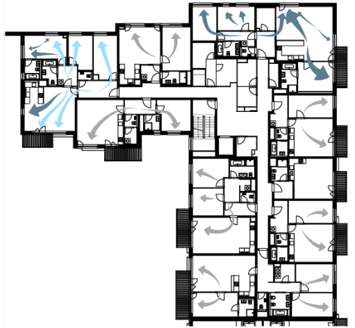
Figure 4.12 Residential Block 4BLOK natural ventilation on 2 nd floor of Block I (source: author)
