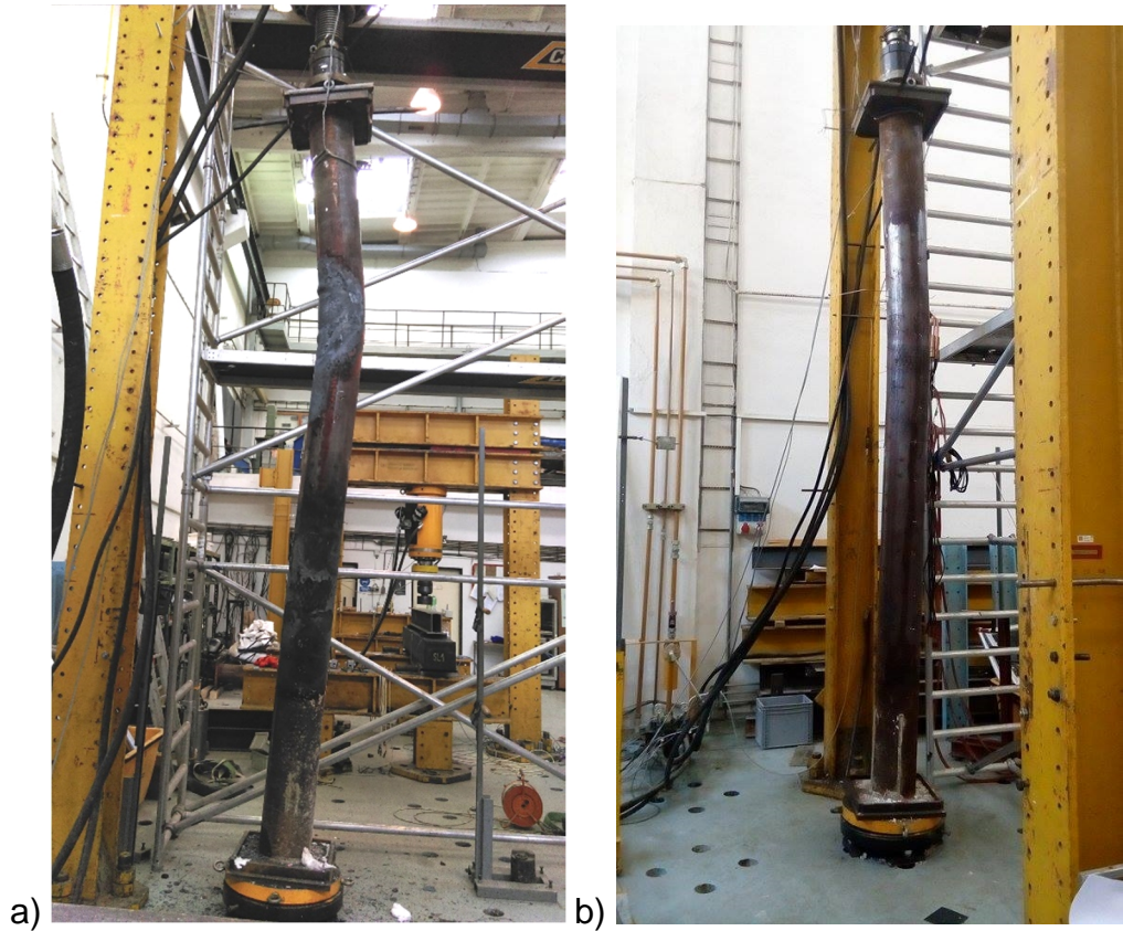
Figure 4-10 - Fail of the tested specimens a) local buckling of the CT1 b) global buckling CT4.
