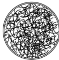
Figure 1-2 Concrete core with steel fibre reinforcement
