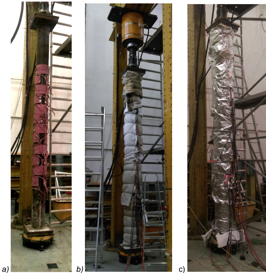
Figure 4-6 – Photo of specimen a) with installed ceramics pads before insulation b) after insulation c) with extra foil installed
