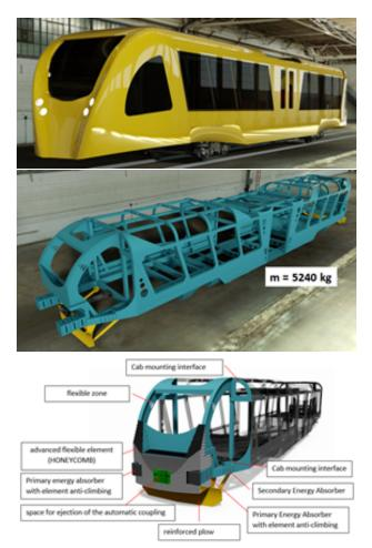
FIGURE 7. Design study of the Rail – electric bus [5].
