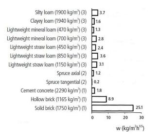
FIGURE 5. Water Absorption Coefficient for earth mixture in literature [3].
