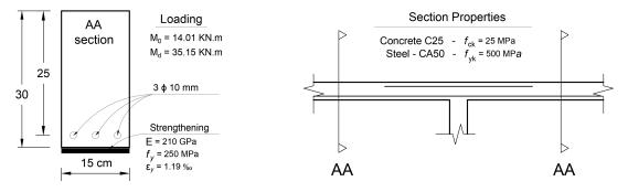
FIGURE 4. Representation of beam characteristics of the building.
