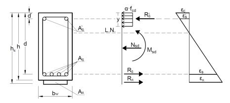
FIGURE 2. Stress and strain diagram for a section in the strengthened condition.
