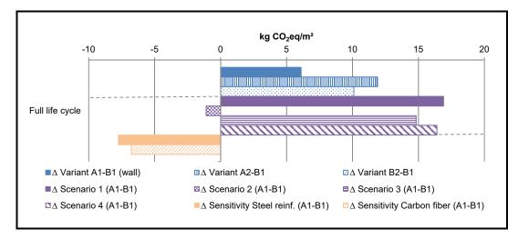
FIGURE 5. Difference in GW scores between wall system variants A (SRC) and B (CCC) for full life cycle of design variants, scenarios, and sensitivity analyses (own illustration).
