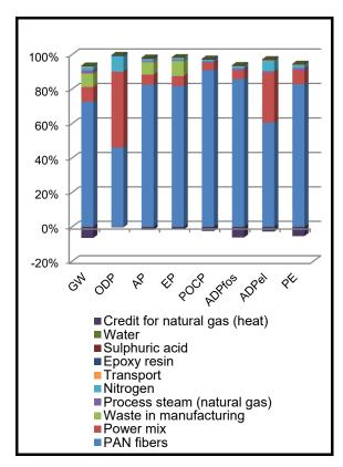
FIGURE 1. Hotspot analysis cradle-to-gate for carbon fiber fabric (own illustration).
