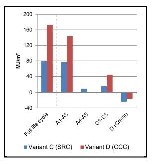
FIGURE 4. Comparing PE scores for ceiling slab reinforcements (own illustration).
