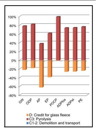
FIGURE 2. Hotspot analysis of the end-of-life stage for carbon concrete (own illustration).
