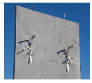
FIGURE 3. Storey-high façade element with new fixing system for carbon reinforced concrete.
