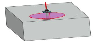
FIGURE 5. Stress distribution in uncracked concrete.
