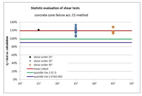
FIGURE 12. Test results vs. calculation results of multidirectional fixing.
