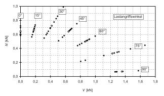
FIGURE 8. Load capacity depending on the relation between axial / lateral load, (DAfStb 2008).
