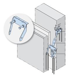
FIGURE 10. Fixing system for façade panels.
