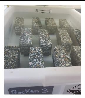
FIGURE 3. Concrete specimen in a storage tank with sulfuric acid.
