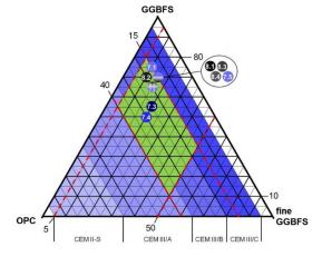
FIGURE 10. Optimized binder compositions for acid resistance tests.
