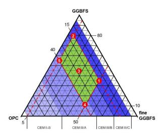
FIGURE 1. Testing area of the binder compositions.
