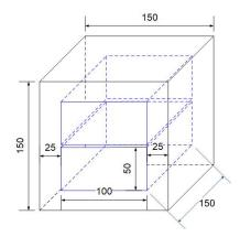
FIGURE 5. Preparation outline of the concrete specimen for acid storage.
