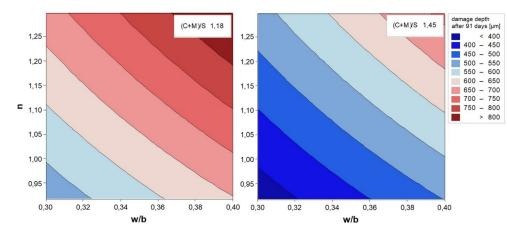
FIGURE 11. Influencing factors to the damage depth of the concrete specimen after 91 days of storage in sulfuric acid.
