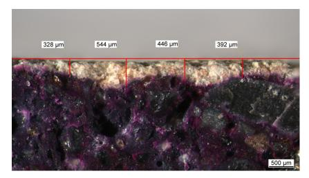
FIGURE 8. Microscopic image of a concrete specimen after 91 days of storage in sulfuric acid.
