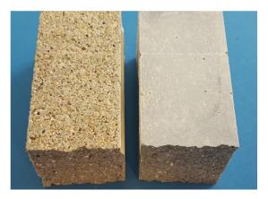
FIGURE 4. Mortar specimen after 91 days of storage in water (left) and sulfuric acid (right).
