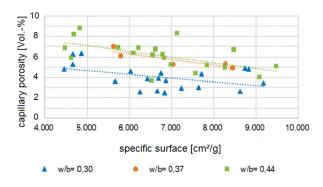
FIGURE 9. Impact of w/b ratio and specific surface on the capillary porosity.
