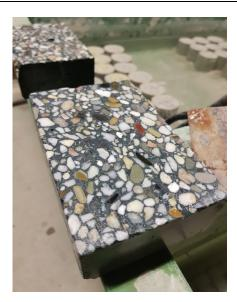
FIGURE 6. Concrete specimen with high packing density of the coarse grain.
