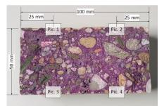
FIGURE 7. Position of the microscopic pictures on the fracture surface of an acid-stored test specimen after spraying on the phenolphthalein solution.
