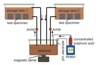
FIGURE 2. Schematic sketch of the acid test rig.
