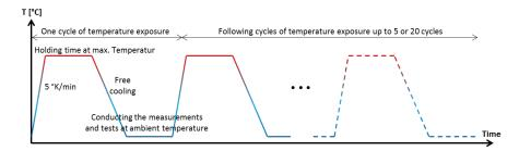
FIGURE 1. Sketch of the heating program, each complete cycle having a duration of 24 h.
