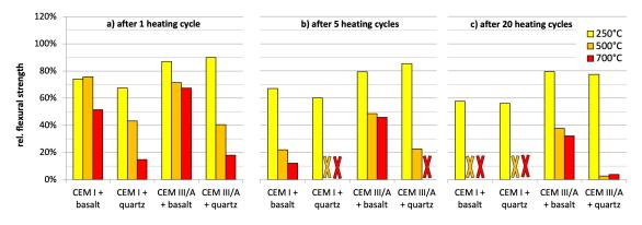
FIGURE 5. Residual flexural strength of the concretes after 1 cycle (a), 5 cycles (b) and 20 cycles (c).
