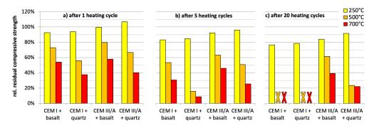
FIGURE 2. Residual compressive strength after 1 heating cycle (a), 5 heating cycles (b) and 20 heating cycles (c). Crosses (X) denote untestable mixtures due to complete degradation.
