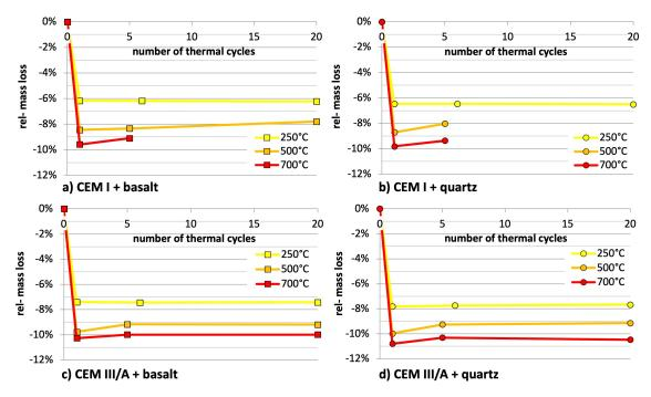
FIGURE 6. Mass loss induced by cyclic heating for all tested concretes.
