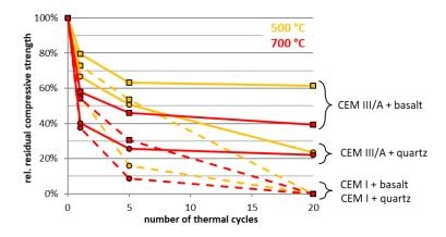
FIGURE 4. Combined effects of type of cement and aggregate on the residual compressive strength after cyclic heating with maximum temperatures of 500  $^{\circ}$ C and 700  $^{\circ}$ C.
