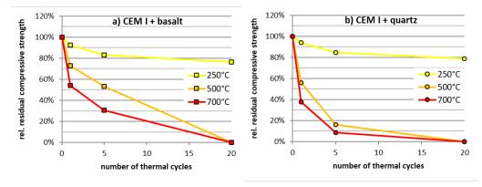
FIGURE 3. Residual compressive strength for concrete containing CEM I and basalt (a) and quartz (b).
