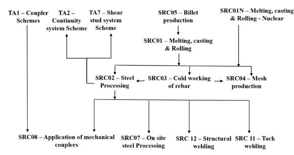
FIGURE 1. Concept of 'extended' product responsibility applied to reinforcing steel.
