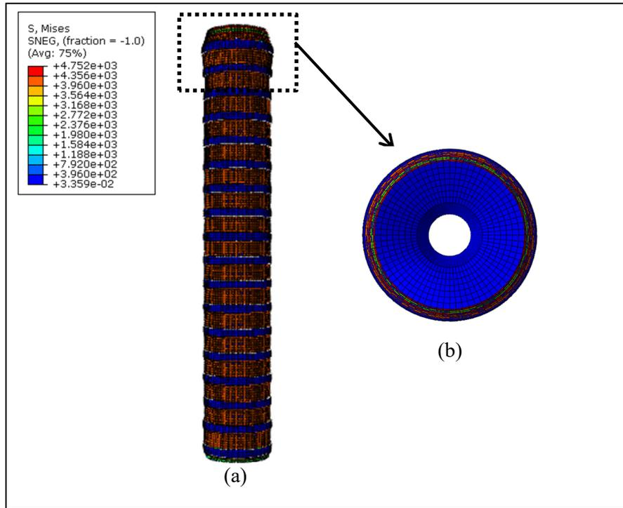
FIGURE 8. Predicted von Mises stress of circular hollow confined RC column strengthened with partial CFRP sheet (at the end of simulation analysis); (a) Front view (b) Upper plan view showing failure behavior on top of the column.
