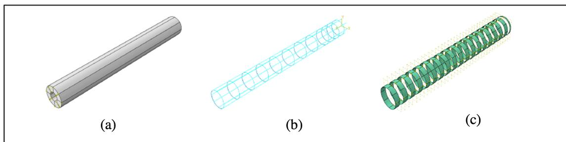
FIGURE 1. ABAQUS FEA model; (a) concrete model (b) reinforcement model (c) CFRP sheet model.
