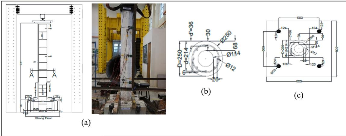
FIGURE 2. Circular hollow unconfined RC column detail specification; (a) Front view (b) A-A section view (c) Plan view [2].
