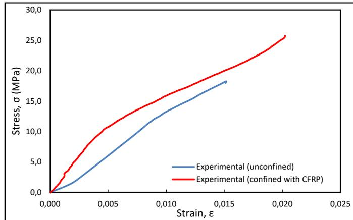
FIGURE 5. Stress-strain relationship of circular hollow unconfined and confined RC column with CFRP under full axial load.
