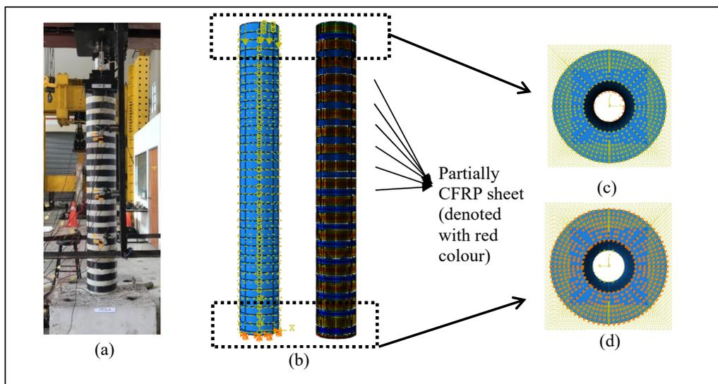
FIGURE 4. Circular hollow confined RC column strengthened with CFRP sheet experimental set-up and modeled in ABAQUS FEA; (a) Front view from experimental set-up (b) Front view (c) Upper plan view showing full axial load imposed on top of the column (d) bottom plan view showing support boundary condition.
