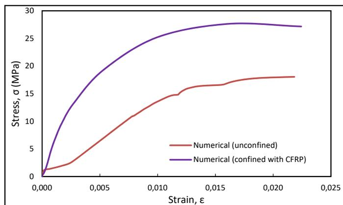
FIGURE 6. Predicted stress-strain relationship of circular hollow unconfined and confined RC column with CFRP under full axial load.
