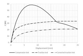
FIGURE 2. Graphs of the course of loading tests of a micropile.
