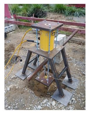
FIGURE 7. Installation of the traction rig at micropile traction load test.
