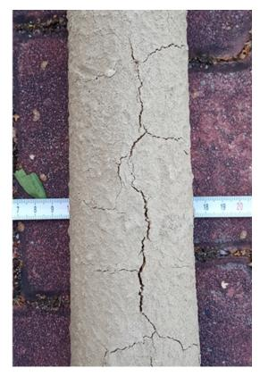
FIGURE 8. The state of the tube shape surface of the micropile after being pulled out of the ground.
