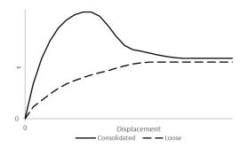
FIGURE 1. Diagram of box shear tests.
