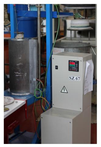
Figure 2. Burst-test experimental apparatus
