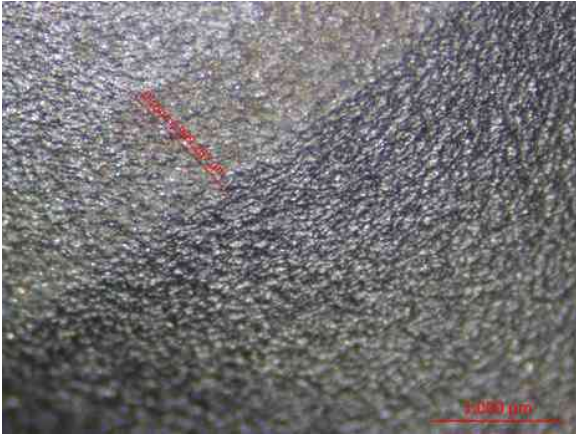
FIGURE 3. Cr CS coated pressure tube - detail of the bottom weld.
