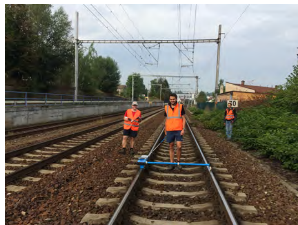
FIGURE 2. Investigation of rail corrugation by the Salamander device - Havlickuv Brod
