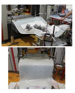
FIGURE 7. Breakdown of the glass railing element.
