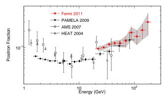
**Figure 4:** Positron fraction measured by the Fermi LAT and by other experiments [32, 33, 17]. The Fermi statistical uncertainty is shown with error bars and the total (statistical plus systematic uncertainty) is shown as a shaded band.
