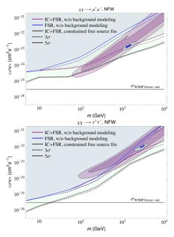
Figure 1: Derived 95% C.L. upper limits on WIMP annihilation cross sections in the Milky Way halo, for the muon (*left*) and tau (*right*) annihilation channels. The purple and blue contours show PAMELA and Fermi positron excess DM interpretation constraint regions.
