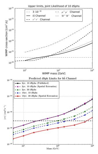
Figure 2: Derived 95% C.L. upper limits on WIMP annihilation cross sections for different channels. *down:* Predicted 95% C.L. upper limits on WIMP annihilation cross sections in 10 years for *bbar* channel.
