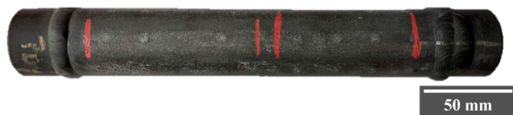
Fig. 1. Tube specimen with welded caps, state after long-term annealing
