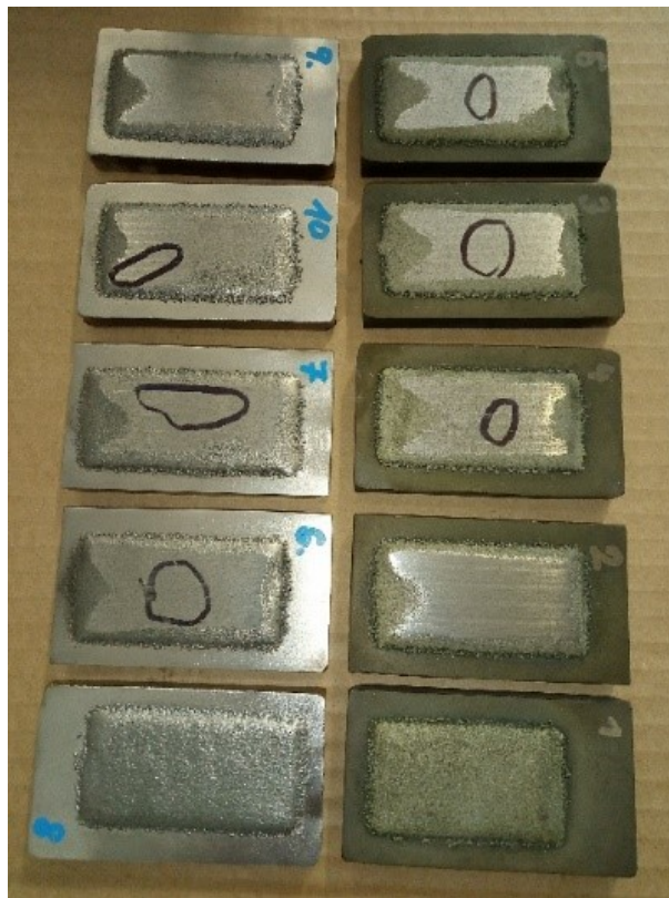
Figure 4.17: Parts polished and prepared for tribology test
