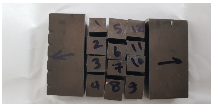
Figure 4.24: Cutting disk with cutting machine square shape (1 cm 2 )
