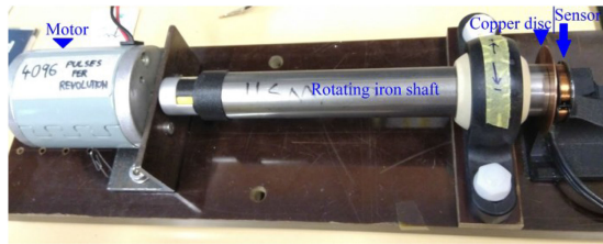
Fig. 11. Experimental elements with dc motor as a prime mover– with rotating iron shaft and copper disc and axial airgap eddy current speed sensor.
