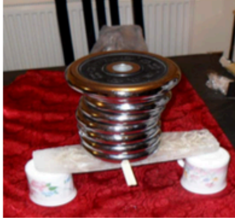
Figure 4: ice beam (2) – reinforced beam supporting a load of 11.25kg
