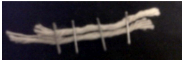
Figure 1: Stapled reinforcement string used in ice beam (2)
