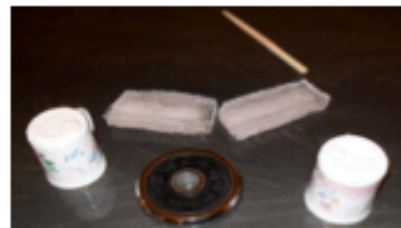
Figure 3 – Ice beam (1) failed under load of 1.25 kg
