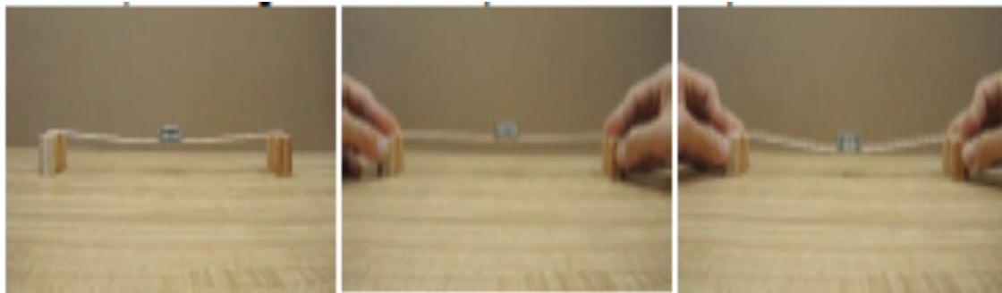
Fig. G2.8.4 Observing combined stresses in beams: (left): flexure only, (middle): flexure + tension, (right): flexure + compression
