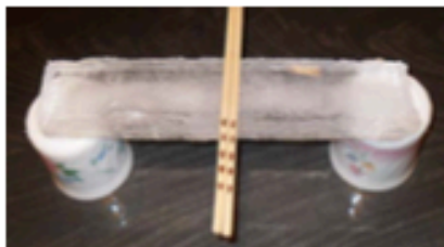
Figure 2- unreinforced ice beam(1)
