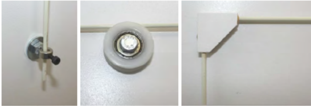
Fig. G1.12.1 Pin joint (left), rolling support (centre) and a rigid corner (right) in comb. with 3 mm GFRP rods
