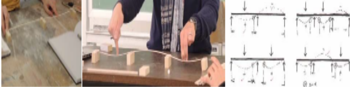
Fig. G2.8.3 Observing deflected shape on continuous beam with 3 or 4 supports.
